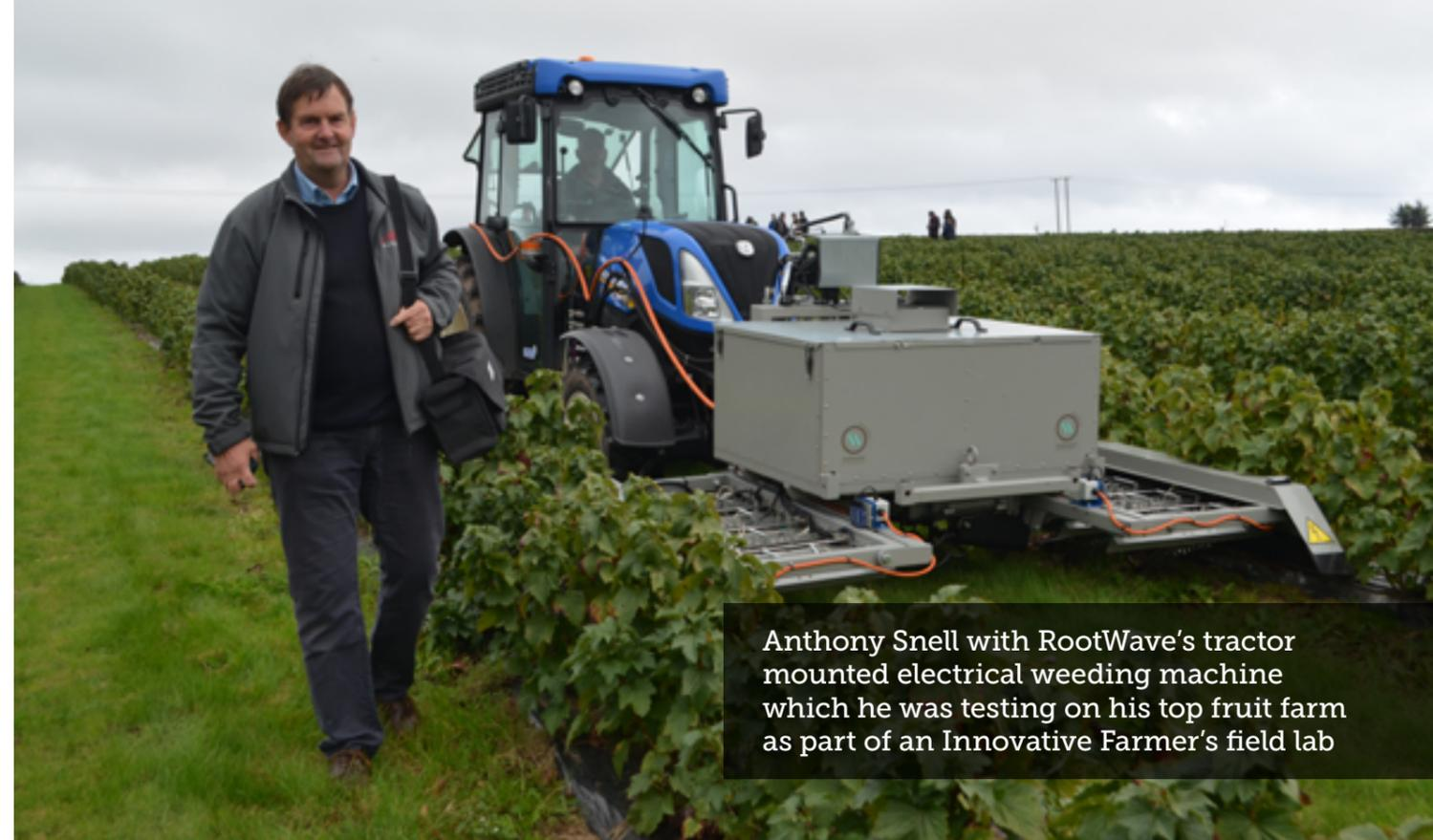
Anthony Snell with RootWave's tractor mounted electrical weeding machine which he was testing on his top fruit farm as part of an Innovative Farmer's field lab
