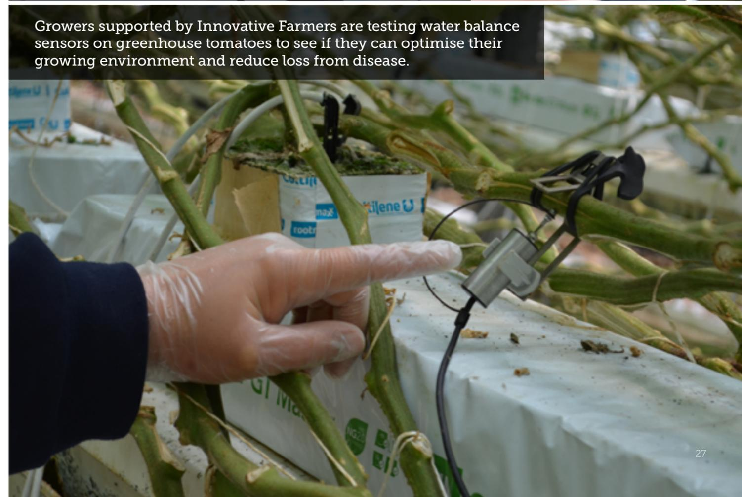
Growers supported by Innovative Farmers are testing water balance sensors on greenhouse tomatoes to see if they can optimise their growing environment and reduce loss from disease.
